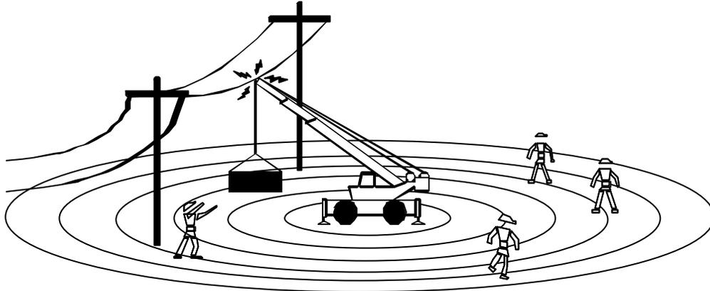
Current can flow outward through the ground in a ripple pattern from the equipment in contact with a power line.
