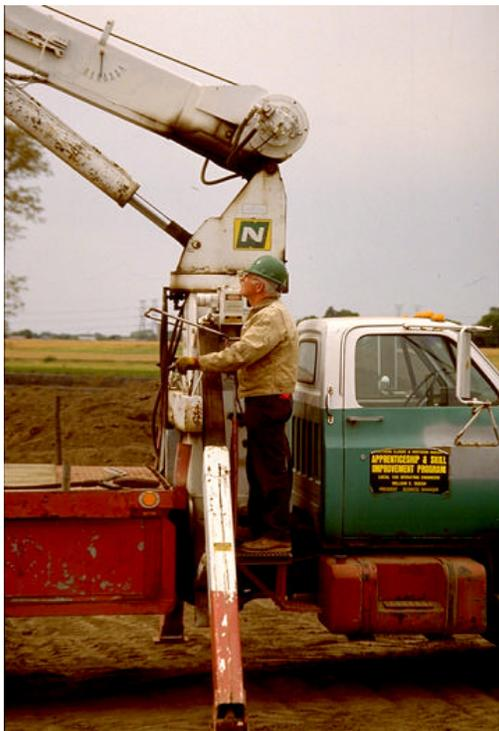
Some manufacturers offer boom truck designs which place the operator on an elevated platform, isolated from the ground.
