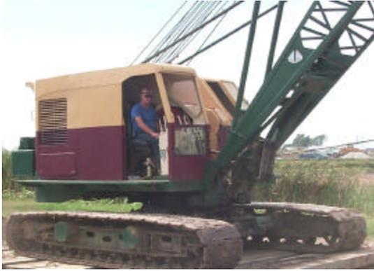
When a mobile crane contacts a power line, the rigger or ground crews are most likely to be affected. The operator sitting in the cab is at the same electrical potential as the equipment.
