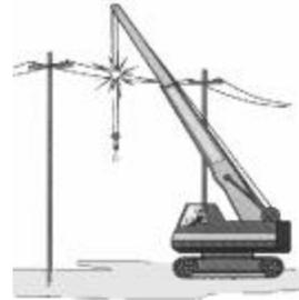
If a power line contact occurs, the operator should stay on the equipment. Don't leave unless there is an extreme emergency.
